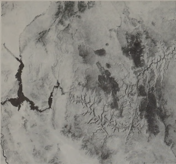
A Landsat image such as this one is used to detect change or surface disturbance. The darker grey is vegetation, black is water. Where there had been surface disturbance, the vegetation pattern would show change on a Landsat image from previous images. When a disturbance is detected, aerial photographs are used to zero in on an area.
